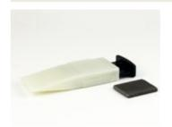
The Combination Planer consists of the modified Special Fillers Applicator with integrated mini Metal Planer blade. This combination tool levels all kinds of König fillers. 90 degree inner edges can be treated not only with the blade of the Metal Planer but also, thanks to an altered groove direction, with the body of the Special Fillers Applicator.
